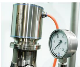
The single cable connection technology of the servo motors provides many advantages, from a hygiene point of view.
