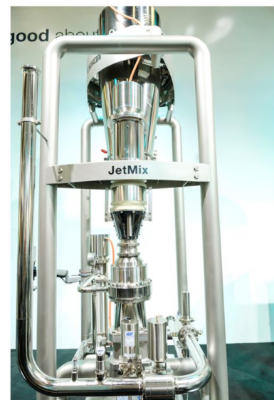
Bühler's JetMix processes flour and water into a smooth pre-ferment. Pre-ferments are common elements of recipes in bakeries. Sourdough from rye flour is one of the most well-known substitutes.
